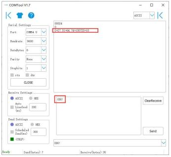
Use extended measurement command 0M1! to read minimum wind direction, maximum wind direction, average wind direction, minimum wind speed, maximum wind speed, average wind speed. The device responds with "00056", which means that the "0M1!" command takes 5 seconds to measure and returns 6 measured values. After 5 seconds, the device responds with its own address "0", indicating that the measurement has been completed.
