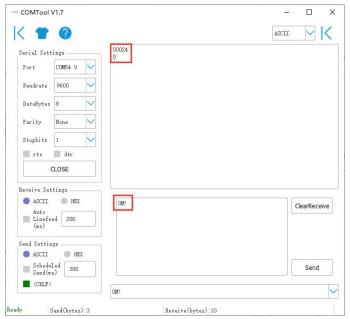
Then send "Read measurement value command 0D0!" to get the 4 measured values of this measurement, which are air temperature  $+27.01^{\circ}$ C, air humidity 64.74%, barometric pressure 100720Pa, and light intensity 10Lux.
