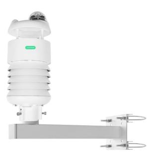
IOT-S300WS7 is an ultimate all-in-one RS485 Modbus weather monitoring system for various and continuous atmospheric conditions including air temperature, relative humidity, barometric pressure, light intensity, rainfall (optical), wind speed, and wind direction (ultrasonic). It boasts high resolution and accuracy with rugged and aesthetic housing.
